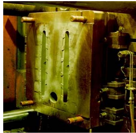
Fig. 1. Fixed half of the investigated die-casting die.
