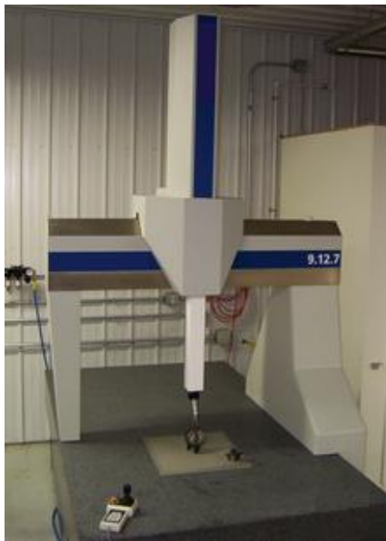
Fig.6 Dimensional metrology using CMM.
