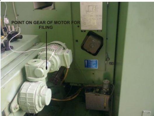
Fig. 3. Side of the machine (a) and motor gear for chip transporter (b)
