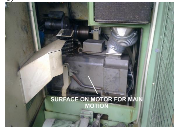
Fig. 4. Motor for hydro-aggregate (a) and motor for the main motion (b)
