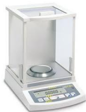
Fig. 4: The scale at which conducts gravimetric analysis of filters.
