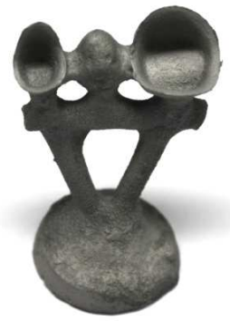
Fig. 8. Casting made construction with casting channels and feeders
