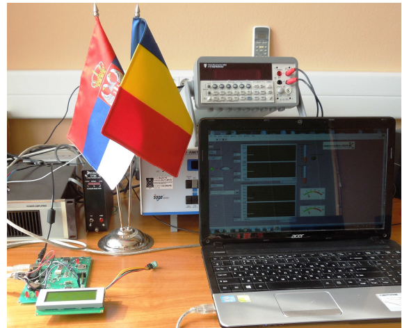
Fig. 6. Hardware outcome of device for indoor and outdoor temperature and relative humidity monitoring
