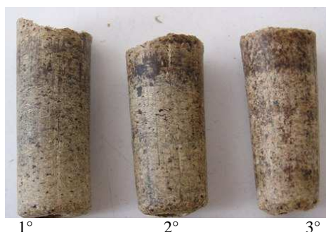
Fig. 10. Negatives of internal chamber space representing different geometries
