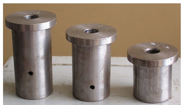
Fig. 5. Cylindrical shaped pressing chambers with various length
