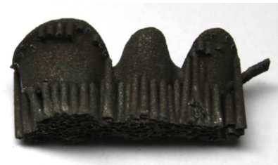
Fig. 10. SLM made construction with support structure
