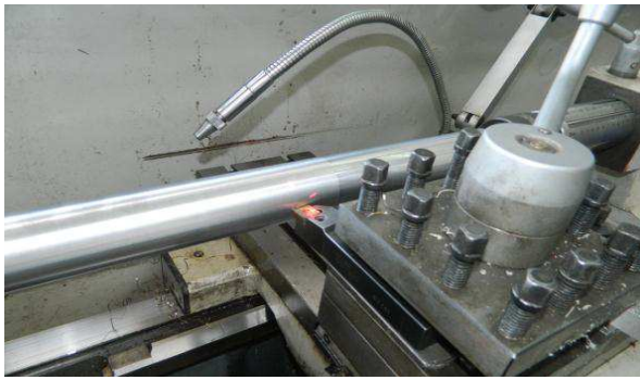
Fig. 8. The turning process of stainless steel material
