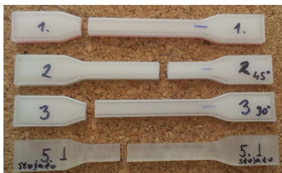
Fig. 6. Tensile test specimens from FDM printer
