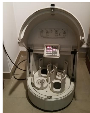
Fig. 3. Planetary ball mill used for mixing and milling of nano powder
