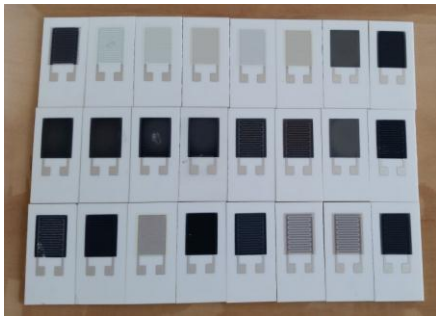
Fig. 6. Screen printed sensitive layer after sintering in furnace
