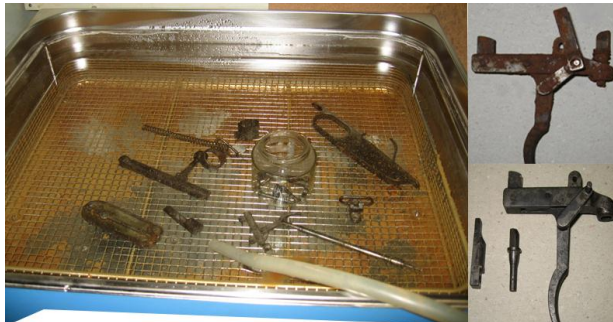
Fig. 4. Ultrasonic cleaning in water
