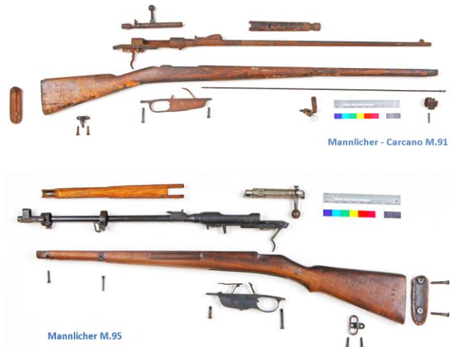
Fig. 3. Rifles separated by components; M91 (above), M95 (below)
