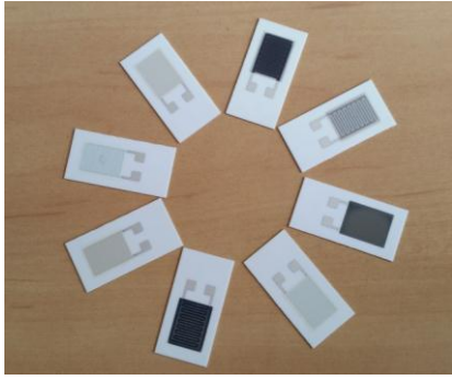
Fig. 5. Screen printing of IDC electrode system and sensitive coatings
