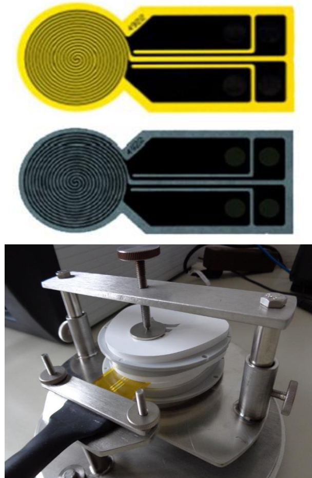
Fig. 2. Sensor element (yellow-Kapton, gray-Mica) (left), sensor sandwiched between two halves of a sample during measurement (right).
