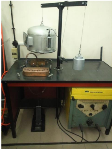
Fig. 1. Photography of the electric-arc furnace for melting and casting
