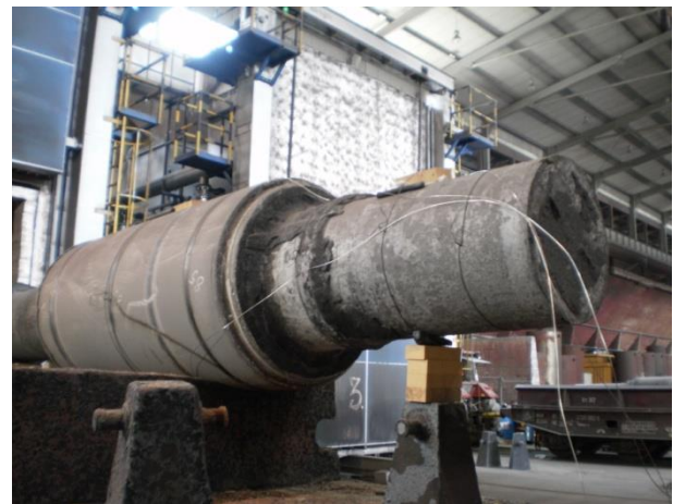
Fig. 7. Protection against sagging.
