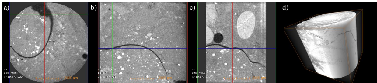
Fig. 1. CT images of the sample "P" scanned with the resolution of 7 \mu m per pixel: cross-section slices (a, b and c) and a volumetric view (d).
