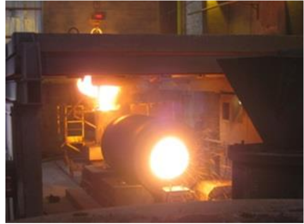
Fig. 2. Centrifugal casting of the working shell.
