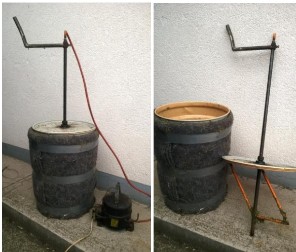
Fig. 2. The laboratory bioreactor
