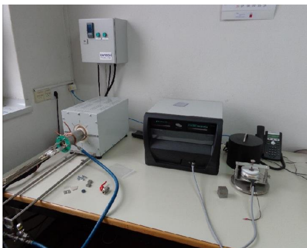
Fig. 3. Hot disk TPS 2200 for measurements of thermal properties
