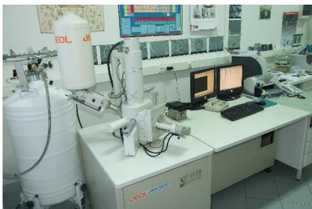
Fig. 2: Scanning electron microscope Jeol JSM 5610 with attached EDS detector
