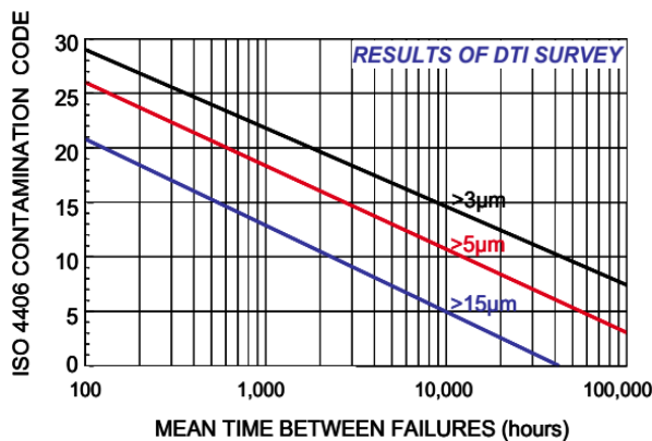
Fig. 3 Ratio of impurity and reliability hydraulic system (Source: UK Ministry of Trade and Industry (DTI))
