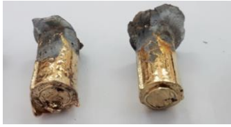
Figure 1. Photograph of casted Cu-Al-Mn-Ni ingots
